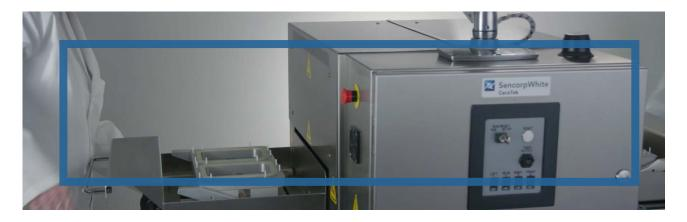
With tray sealing, a flexible material (lid) is bonded to a rigid material (tray).
