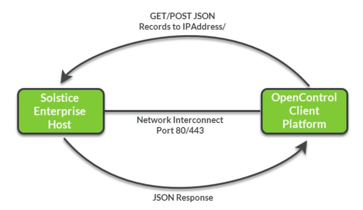
OpenControl operates over existing TCP/IP network infrastructure to allow third-party client platforms to control and query Solstice endpoints. The protocol is based on a REST architecture that encapsulates communication into independent GET/POST events, sent to particular URLs on the Solstice Pods, each of which result in a JSON formatted response.
