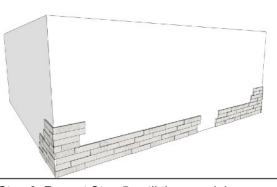
Step 6: Repeat Step 5 until the remaining open space is less than a full Precipice Panel.
