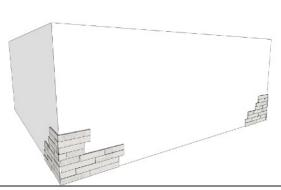
The wall should now appear like the diagram above. The distance between the corners will vary and are project specific.
