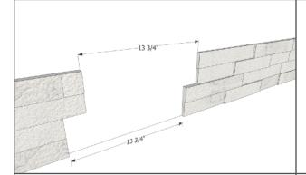
Step 7: Measure the distance between the two full panels as shown. This distance will vary by project.
