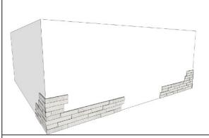
Step 5: Moving inwards from each corner, install Precipice Panels on the face of the wall as shown.
