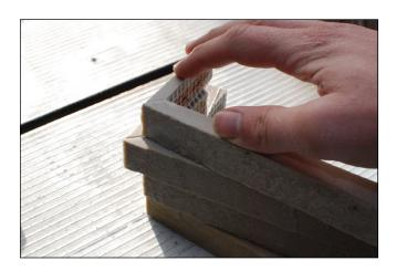
You should now have matching miter pieces to create a desired miter joint with the rustic cladding.
