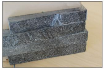
Pay special attention to the positioning of each piece of cladding while installing so they do not move as this relates to the other pieces in the set and will affect the tightness of the interlock with the next piece of cladding.
