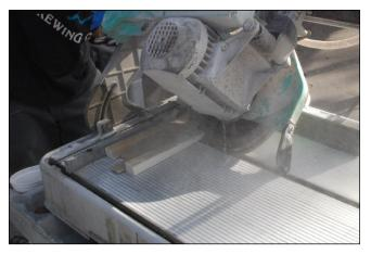
**Step 4.** With saw positioned at desired angle (45° shown), hold tile flat against tray surface and guide while making the first miter cut.
