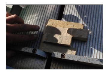
**Step 5.** Remove first miter cut piece and turn remaining piece 180° around and reposition so that saw will cut 2nd matching miter cut. Important! Piece should be positioned so that saw cuts as close as possible to the highest piece of the side being cut.
