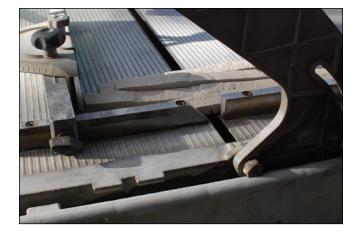
**Step 3.** When making cuts, cladding piece should always be placed with the bottom of the cladding against the tray guide. All pieces should also be flat on the saw's tray.
