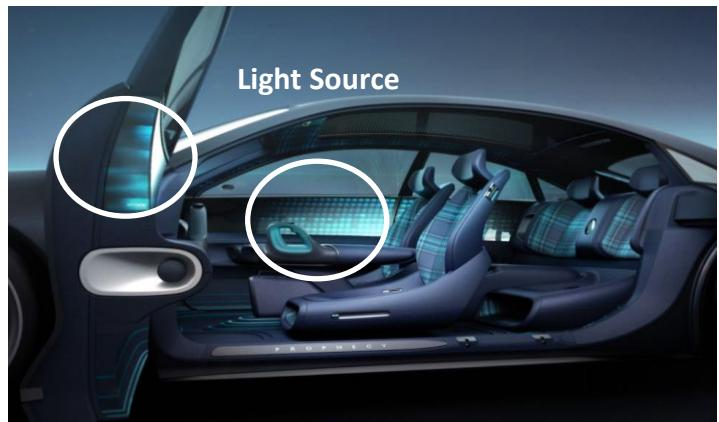
*Metocene HM840N* is a very transparent resin, metallocene-based, homopolymer used for Automotive compounding. *Metocene HM840N* also has good stiffness and gloss, so it is used for LED beam housing in automotive door trim, console parts.
