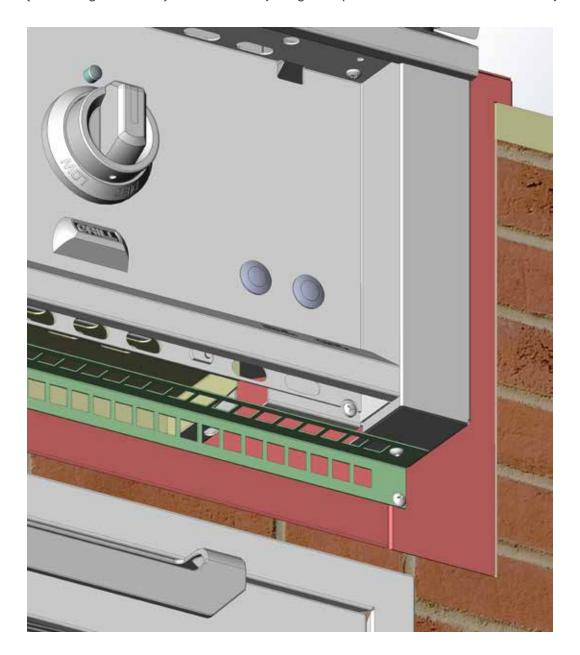
8. Proceed with the remainder of the grill installation as documented in the Use & Care Manual that came with your Hestan grill. Follow all instructions for regulator installation, gas connections, leak testing, burner adjustment, etc. before using your grill. After all these steps are completed, you can re-install the control panel and knobs.
