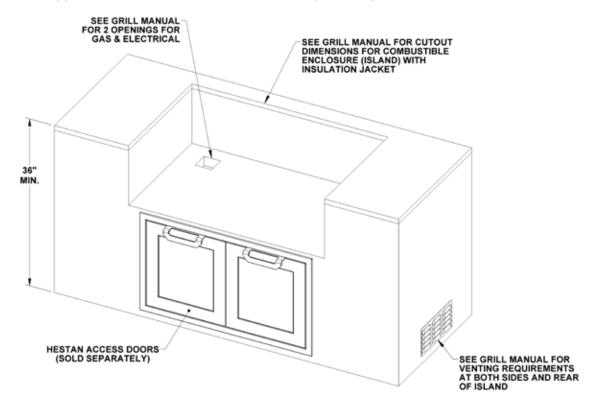
2. Slide in the Insulation Jacket as per the image below. The front face of the jacket should be flush to the face of your island.
