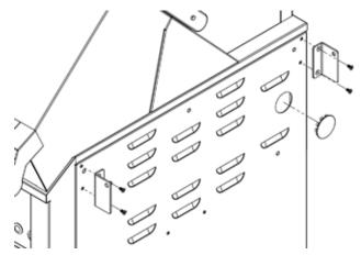
3. Install the front of the shelf on the front pin, then tilt the rear of the shelf up to meet the threaded hole at the rear bracket and install the hex bolt with a 7/16" wrench or socket wrench.
