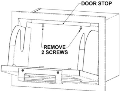
3. Slide the frame into the opening and check for proper alignment. Secure the frame to the structural members of your island using the slotted mounting holes as shown below. Open and close the door several times to check for proper function. Replace the door stop and 2 screws.
