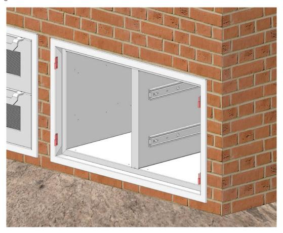
4. Reinstall the drawer(s) by aligning the slides on either side and push the drawer back into the opening. You will hear the release levers click. Open and close the drawer a few times to check for proper function and alignment. There are adjustment screws on either side of the drawer should vertical adjustment be needed. Reinstall the door back onto the pins - there is no adjustment.
