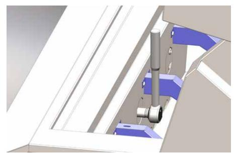
6. If your grill is equipped with both open-flame (Trellis or U-Burners) and Infrared Sear Burners, verify you have the correct orifice for each kind of burner. The orifice size is stamped on the body of the orifice. Consult the chart at the end of this manual for what size is used on each burner type. This is also a good time to clean and inspect the burners for clogged ports, debris, spider webs, etc.
