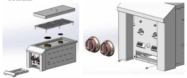
2. Reach inside the burner to hold up the orifice holder against the burner bowl (to prevent it from falling) and remove the 2 Phillips head screws securing the burner base. Continue to hold the orifice holder against the burner bowl and reinstall the 2 Phillips head screws back onto the orifice holder so it doesn't fall.
