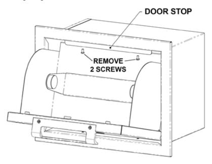
3. Slide the frame into the opening and check for proper alignment. Secure the frame to the structural members of your island using the slotted mounting holes on left and right sides as shown below. Open and close the door several times to check for proper function. Replace the door stop and 2 screws.
