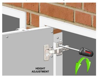
6. The side and depth adjustment of the doors are shown below. Make small adjustments and close the door between each attempt to see how the door looks relative to the frame opening and the adjacent door.
