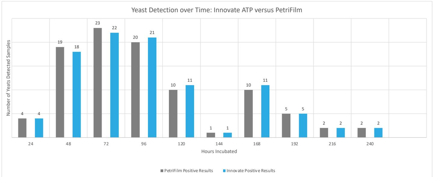
Moreover, the calculated Probability of Detection (%PoD) for the Innovate System ranged from 95-110% over the testing period. Probability above 100% was calculated based on accurate ATP detection of a known contaminant compared with zero detection by PetriFilm, the comparative (traditional) method.
