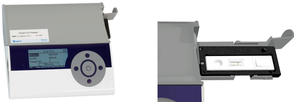
2. When using the Reader in stand-alone mode, enter the identification data of the sample in the device and press "measure" to start the reading. The result will appear on the screen as “ppm of gluten”.
