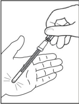
1 A: Allow devices to equilibrate to room temperature. Shake tube by tapping on the palm of your hand 5 times to bring liquid in tube to the bottom of the tube.
