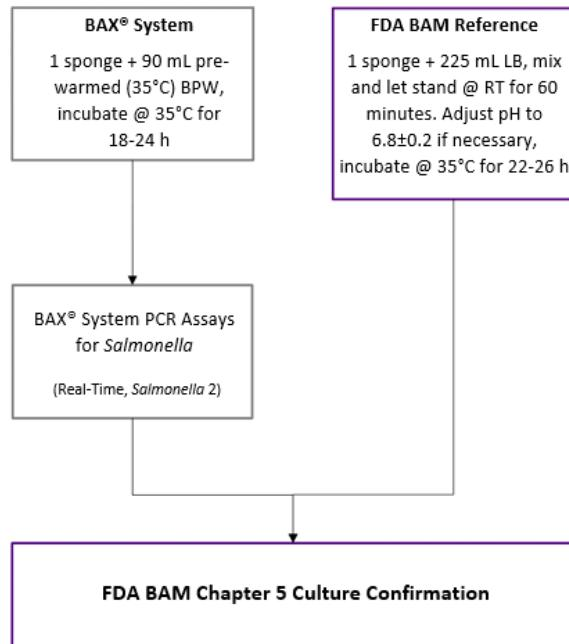
**Figure 1.** Unpaired study to compare the BAX® System method to the FDA BAM reference method for environmental samples.
