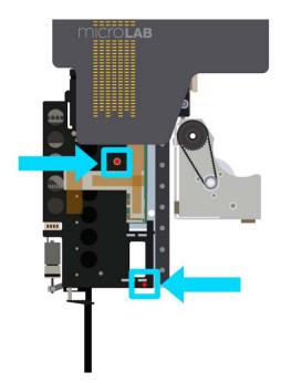
2. **Examine the back of the channel before proceeding to see how the slots and tabs fit on a correctly installed pipetting head.** A pipetting head may "fit" without each of the four tabs lining up properly, which can cause errors later.
