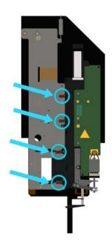
3. **Push the pipetting head removal tool through the indicated hole.** The pipetting head will be ejected slightly.
