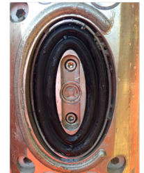
Even with 40 oval pad activations, the GeoTap® IDS sensor is still in perfect condition to take more formation pressure samples.
