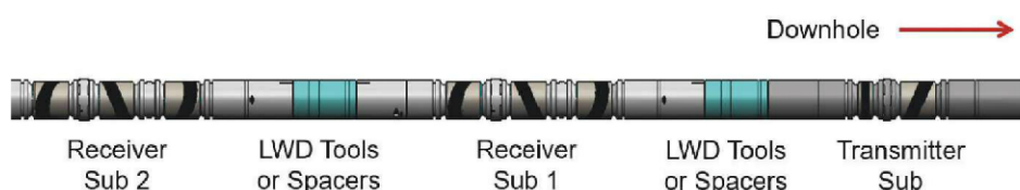
FIGURE 1. This is the basic layout of the EarthStar service tool with the transmitter collar located toward the lower end of the BHA. (Source: Halliburton)
