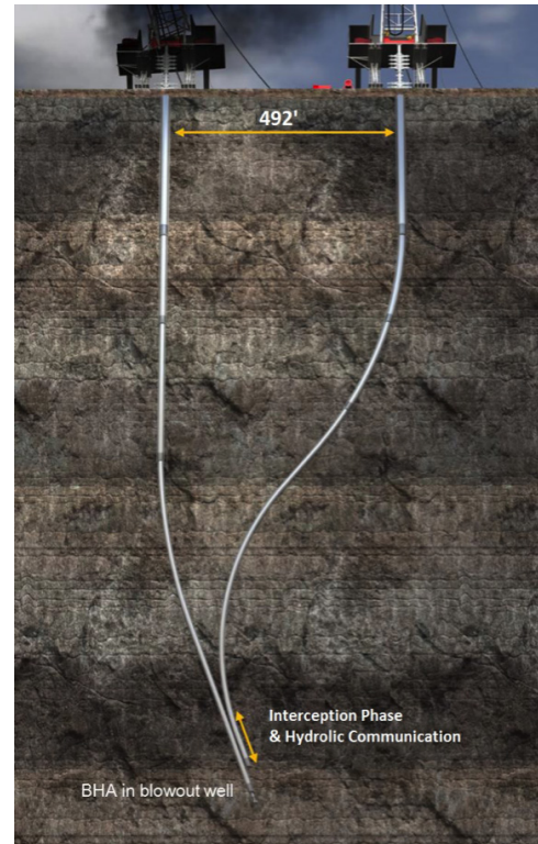
WellSpot™ active magnetic ranging services supplemented by passive ranging services intercepted the target well and relieved the blowout.
