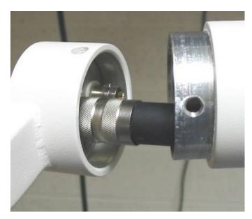
Install the arm cable (six-pinned connector) on the receptacle on the yoke as shown. NOTE: Both the connector and receptacle are keyed. Slide the connector in and then fasten to secure.
