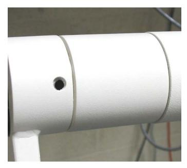
Slide the camera head assembly over the shaft protruding from the arm. NOTE: Pull any cable slack from the wheel-casting end if necessary.
