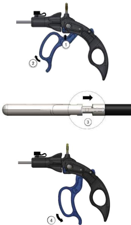
1. With handle in the pistol-grip position, depress the insert release button (G), move trigger (F) fully forward into the eject position.
