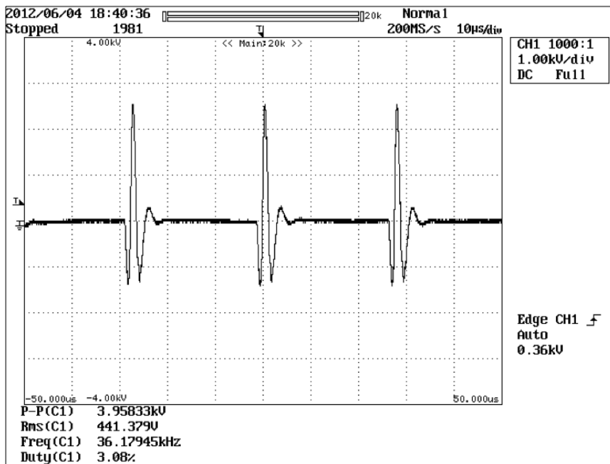
Figure 3– 21 Spray Coagulation Output Waveform (2000 Ohm Load)
