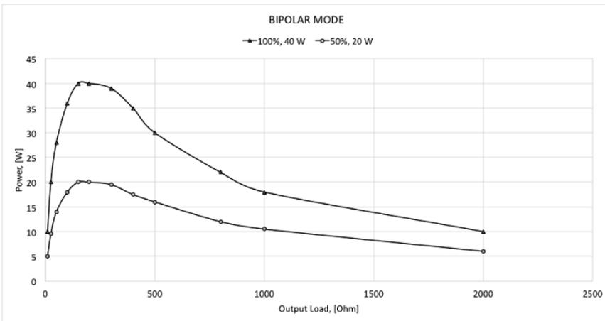
Figure A – 11. Output power vs impedance for Micro Bipolar mode
