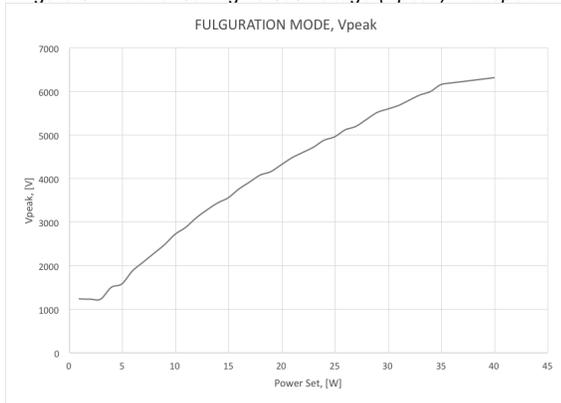
Figure 6 Power setting versus voltage (Vpeak) Bipolar
