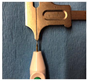
Figure 4: Ultra-thin cautery wire tip (~.07 mm)
