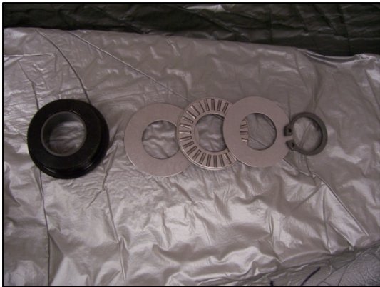
22. Parts to install into Elbow: a. Plastic bearing. b. Thrust bearing components. c. Retaining ring.
