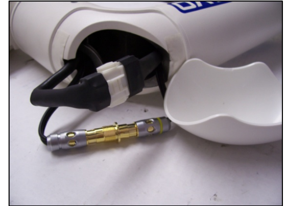
27. Terminating connectors in elbow.
