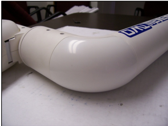
28. Attach elbow cover. Note arrow inside part surface points up.
