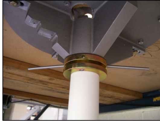
20. Position Rods and tighten Jack Screw.
