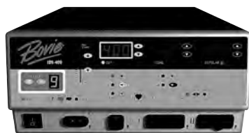
Figure 2 – 2 Controls for setting and recalling presets
