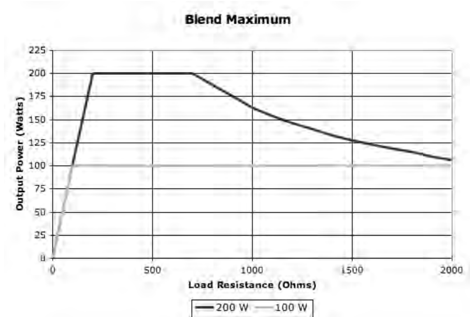
Figure A – 5 Output power vs impedance for Blend Max mode
