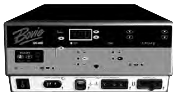
Figure 2 – 7 Location of the unit power switch and front panel receptacles
