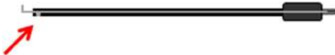
Fig. 6. Insulation failure. Insulation failure is the break of the insulation material along the shaft of an instrument. In this graphic, a laparoscopic L-hook active electrode is depicted with a defect in its insulation. This defect allows stray energy transfer to burn unintended tissue. Of 5 laparoscopic instruments, 1 has been shown to have 1 or more insulation defects. (Adapted with permission from Thomas N. Robinson.) (Color version of figure is available online.)
