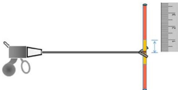
Fig. 5. Direct application. The distance of thermal injury from the instrument tip following an activation represents direct application. In this graphic, the orange area adjacent to the device's jaw represents the distance of thermal spread resulting from energy application. Direct application has been recognized as the most common energy-based device complication pattern. (Adapted with permission from Thomas N. Robinson.) (Color version of figure is available online.)
