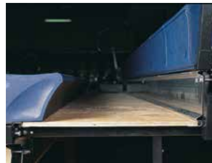
E. Full-Length Captured Decking Decking is captive in the riser beam and rests on the nose, firmly secured by the seat bracket. This system provides a stiff, secure walking surface with no exposed hardware. MAXAM is the only telescopic gym seat that utilizes transverse decking, using decking materials in accordance with their industry span rating. Load tested and independently verified, MAXAM's support system provides an enhanced level of performance, safety and stability.
