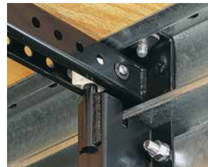
D. Captive Interlock & Adjustable Row Stops The Captive Interlock System engages and aligns deck to deck. In addition, MAXAM® can be configured for three different row-spacing setups—adjustable on-site if required. MAXAM incorporates three stabilizer assemblies per section to provide improved tracking and stability.
