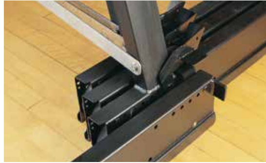
A. Posi-Lock™ LX These automatic row locks prevent accidental closure when the system is in use. This patented, innovative, low-profile design minimizes the chance of accidental damage, ensuring consistent operation.
