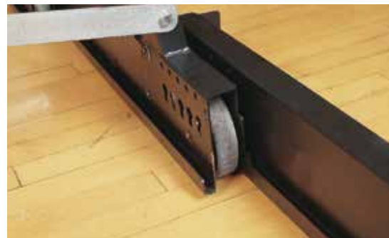
C. Continuous Positive Interglide This interlocking glide system is a rigid, one-piece formed design which tracks better and operates easier than systems with 1/2" (13 mm) row to row engagement. The 10" (254 mm) minimum interlock provides the industry's most rigid, stable design. Our wheels are 5" (127 mm), resulting in less rolling friction.
