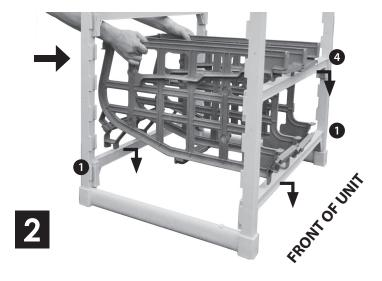
• = Traverse installation position on dovetails
