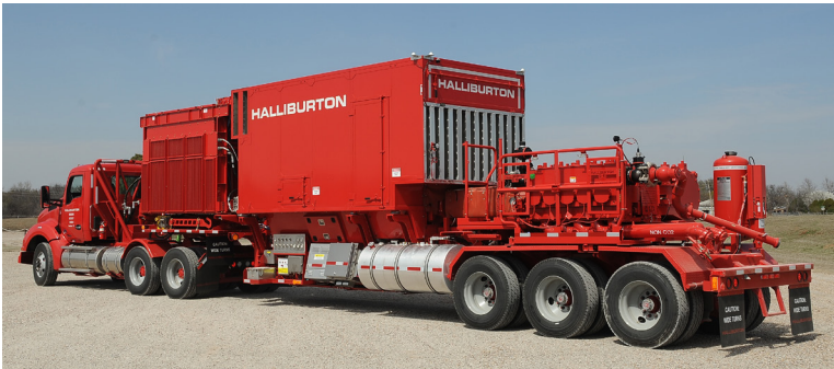
Coupling the advanced Q10™ pump with noise mitigation technology, Halliburton has developed an unconventional pump for sound-sensitive areas.
