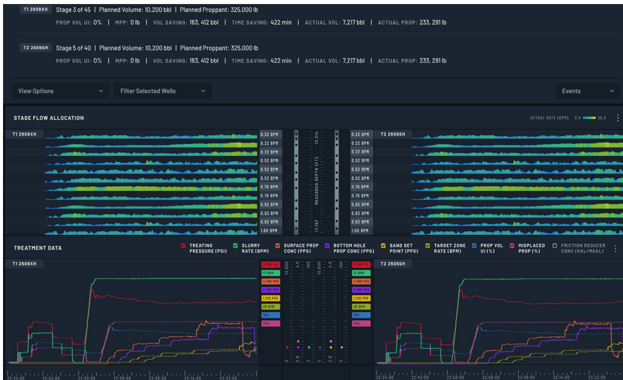
SimulFrac operation: Near wellbore fluid distribution
