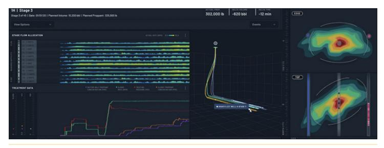
The SmartFleet system provides real-time visualization of fracture measurements, cluster uniformity and well interactions.
