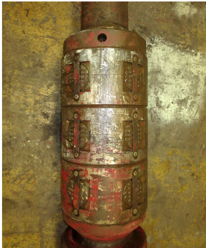
RTTS® packer after being in the well for nine years
