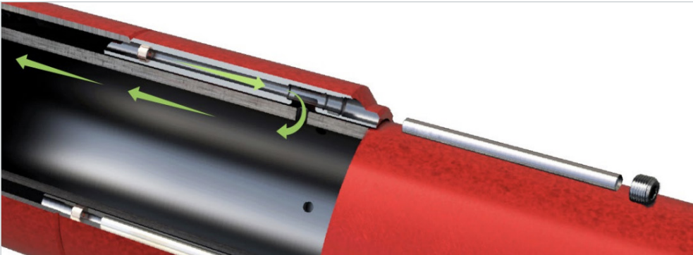
Removing adjustment rod opens nozzle to flow
