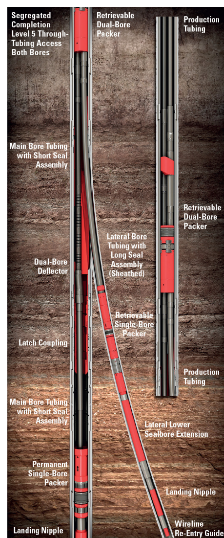
Figure 1: Full isolation of lateral or main bore using through-tubing pressure-isolation sleeve (lateral isolation) or bridge plug (main bore isolation)
