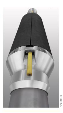
For the cable design, Halliburton provides the installation tool that fits easily on the rotary cable and "zips" the control cable or flat pack through the packer.
