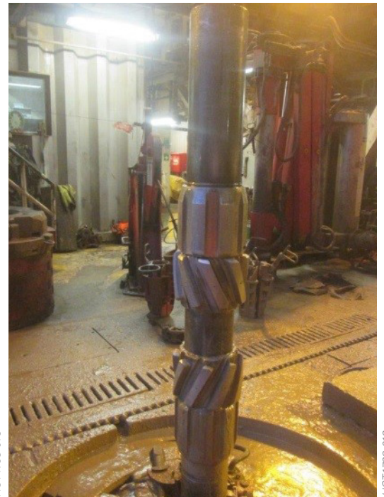
Well No. 2 –The 9 5/8 inch Drill Tech® scraper's condition after drilling 341 meters (1,119 feet) of open hole
