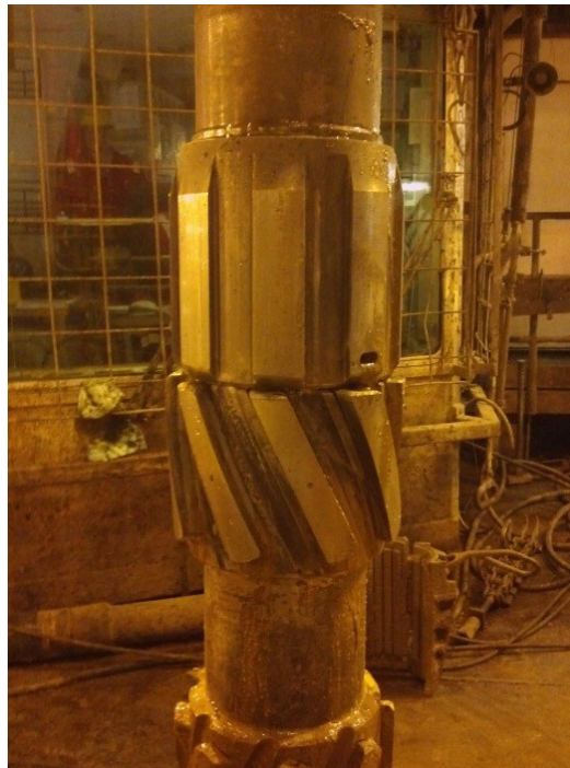
Well No. 1 –The 9 5/8 inch Drill Tech® scraper after drilling tieback, shoe track, and 81 meters (266 feet) of open hole
