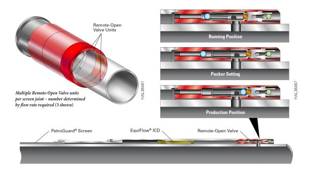
The remotely controlled PetroGuard® screens and EquiFlow® ICDs (Inflow Control Devices) hold internal pressure when closed, but open the screen to full production flow after sufficient internal pressure is applied and released.
