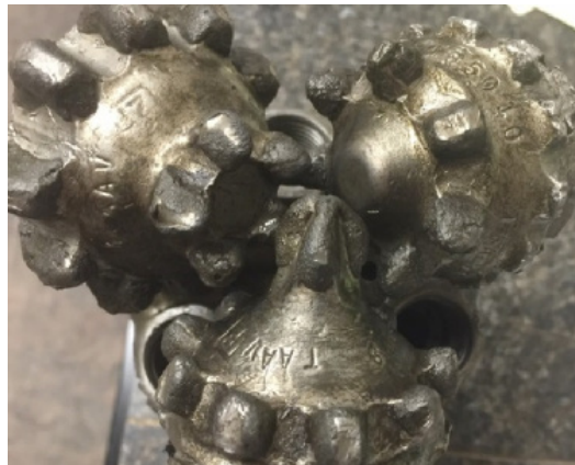
Roller cone Bit #1 - Drilled out 70 Obsidian® frac plugs with no short-trip
