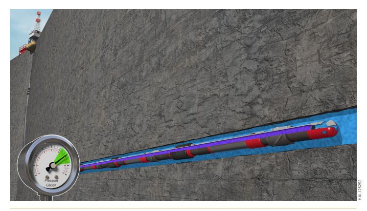
Washpipe-free ICD completion provides washdown, circulation and pressure capability without inner string
