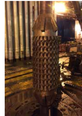
Mag Tech® riser magnet recovers 97.43 pounds of well debris.
