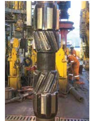
9 7/8-in. Bristle Tech® brush was residue free when pulled out of hole.
