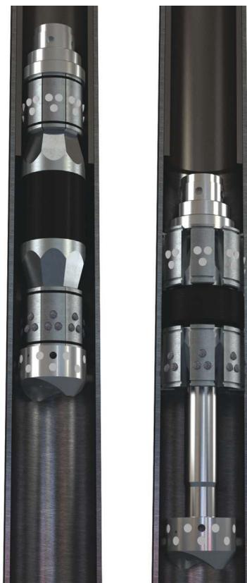
**Illusion® High-Expansion frac plug as it passes through a restricted ID and sets in nominal casing ID, enabling wellbores with restricted IDs to be completed.**
