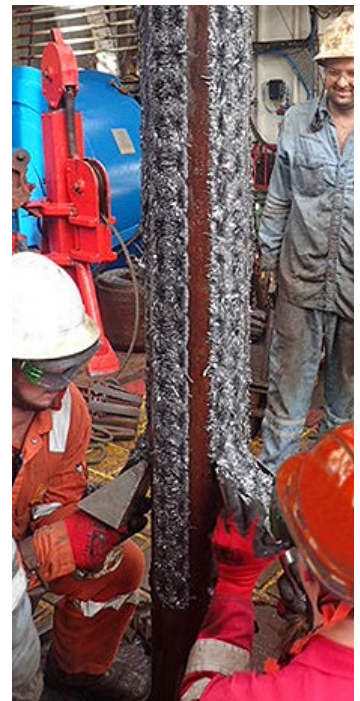
PowerMag® magnet being cleaned on rig floor after milling run with cleaning tool
