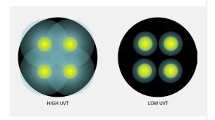
UV Transmittance (UVT) is the ratio of light entering a fluid to that exiting the fluid. Fluids with high UVT allows more UV light to reach the organisms you are trying to treat.
