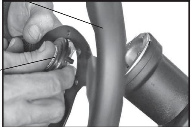
Note: Before steering wheel install, make sure the front tires are straight and in line with the rear tires. Uninstall the 6 - M5X20 allen bolts and clamp ring from the steering column.
