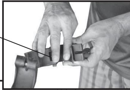
1. Install rubber straps in buckle assemblies for windshield.
