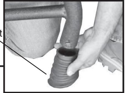
1. While on the ground, place front and rear roll cage boots onto the appropriate bars.
