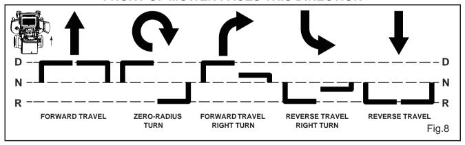
N = NEUTRAL POSITION D = DRIVE POSITION R = REVERSE POSITION Direction of arrows indicate direction of mower movement
