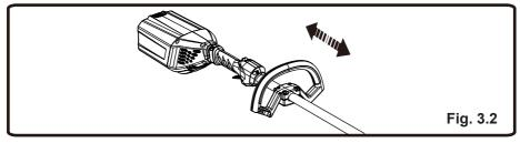
4. Insert and tighten the four screws so that the handle cannot be rotated on the shaft.
