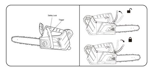
**NOTE:** It is normal for the chain to coast to a stop once the trigger is released.
