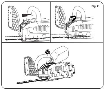
**NOTE:** Chainsaw comes from the factory with no bar and chain oil added. The level should also be checked after every 20 minutes of use and refilled as needed.
