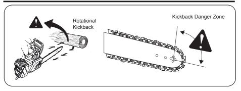
Kickbacks result from incorrect use of the tool and/or incorrect operating conditions or procedures, and can be avoided by taking the appropriate precautions specified below:
