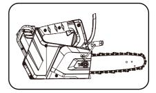
NOTE: During normal saw operation, the temperature of the chain increases. The drive links of a correctly tensioned warm chain will hang approximately 1/16 in. (1,58 mm) out of the bar groove.
