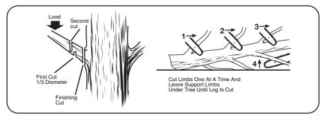
When bucking on a slope always stand on the uphill side of the log. When cutting through to maintain complete control release the cutting pressure near the end of the cut without relaxing your grip on the chainsaw handle. Do not let the chain contact the ground. After completing the cut, wait for the saw chain to stop before you move the chainsaw. Always stop the motor before moving from tree to tree.
